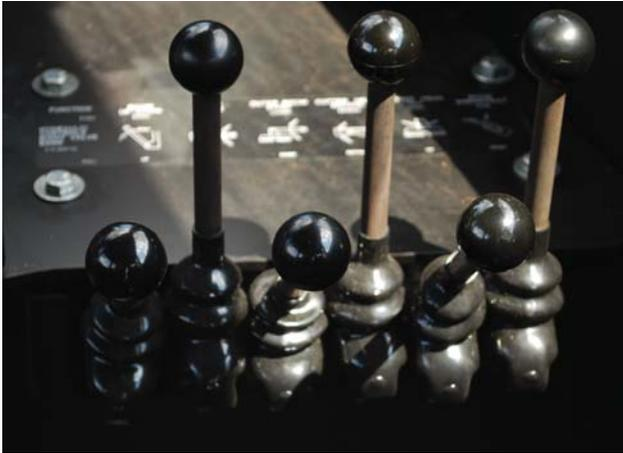
Lever-style operator controls provide precision positioning of the booms and cutter heads.
