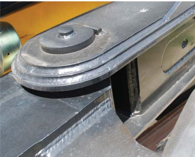
Breakaway boom joint protects boom by rotating backward when encountering an immovable object.
